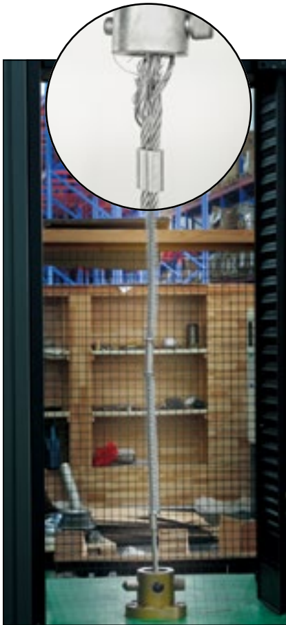
Snatch test to check the maximum straining force of whipcheck cables.
